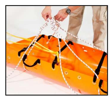
3. TIE FIGURE 8 KNOTS IN BOTH ENDS OF THE ROPE LEAVING ABOUT 2.5 FEET EXTENDING UP FROM THE FOOT END SLOTS AND SHORTER AT THE HEAD END. (SEE PHOTO IN STEP 4)
