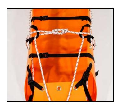
8. TIE AN OVERHAND KNOT ON EACH SIDE OF THE SQUARE KNOT FOR SAFETY.
