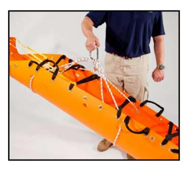
4. THE ROPE AT THE HEAD END MUST BE A BIT SHORTER THAN THE FOOT END TO PROVIDE A SLIGHTLY "HEAD UP" ATTITUDE FOR PATIENT'S SAFETY AND COMFORT.
