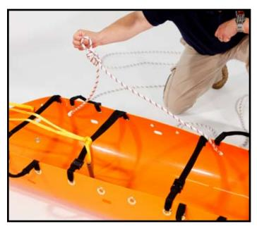
1. HOLD THE PRE-TIED FIGURE 8 KNOT IN THE CENTER OF THE ROPE AND PASS THE ENDS OF THE ROPE THROUGH THE ANGLED LIFT SLING SLOTS FROM THE INSIDE-OUT.
