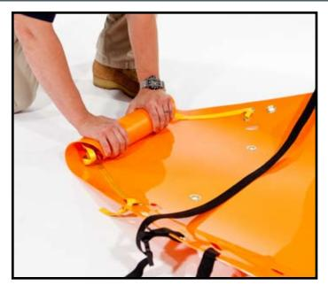
1. LAY STRETCHER OUT FLAT WITH ALL CROSS STRAPS CONNECTED.
