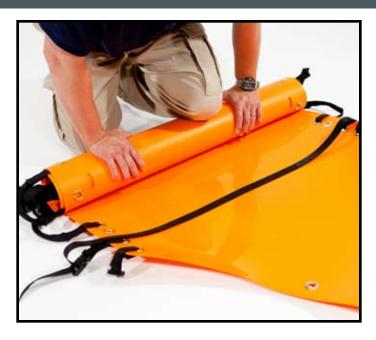
2. STARTING AT THE HEAD END, ROLL THE SKED® UP AS TIGHT AS POSSIBLE. CONTINUE TO ROLL THE SKED® USING KNEE TO KEEP THE ROLLED STRETCHER SMALL.
